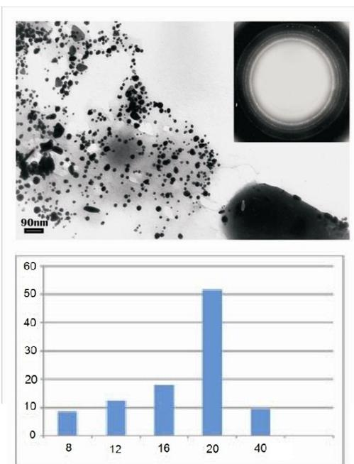
Fig. 1. TEM image and size histogram of Au nanoparticles in biomass of *Arthrobacter 61B*
