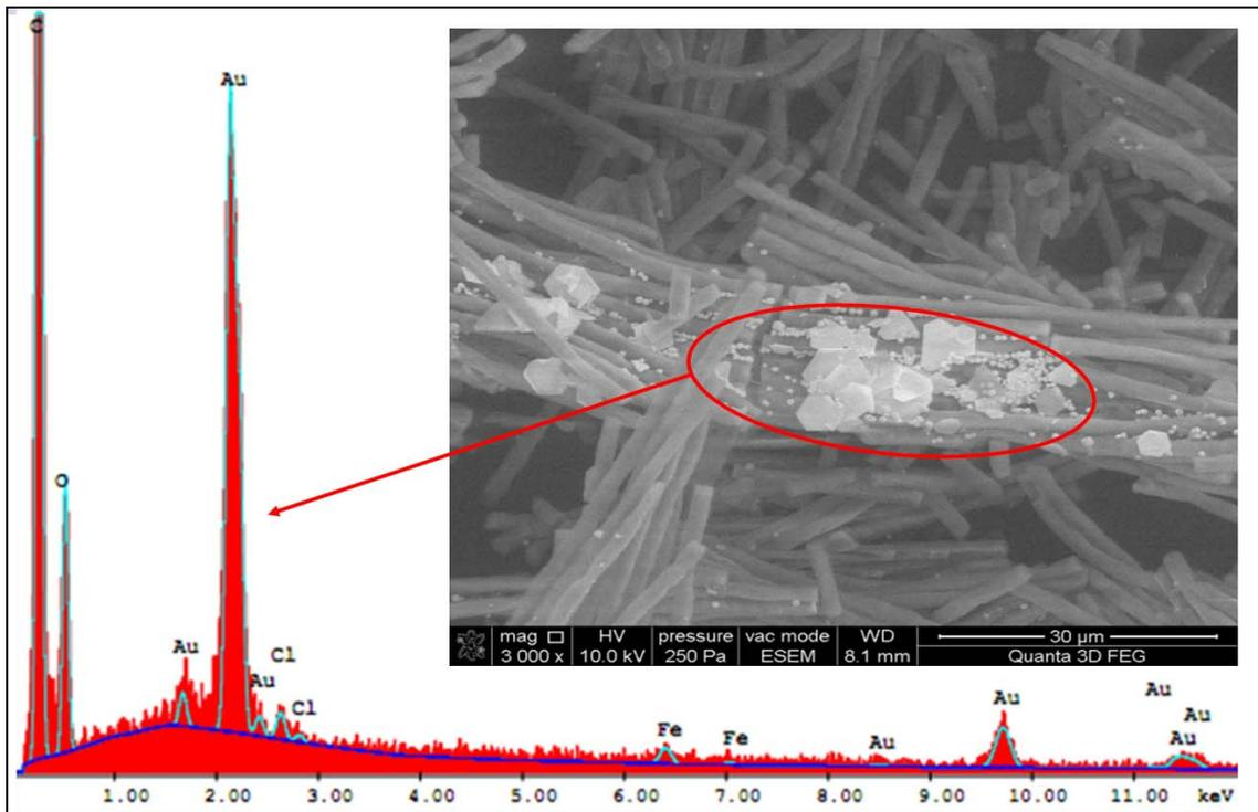
Fig. 3. EDAX spectrum of *Spirulina platensis* exposed to  $\text{HAuCl}_4$  ( $10^{-2}$  M)
